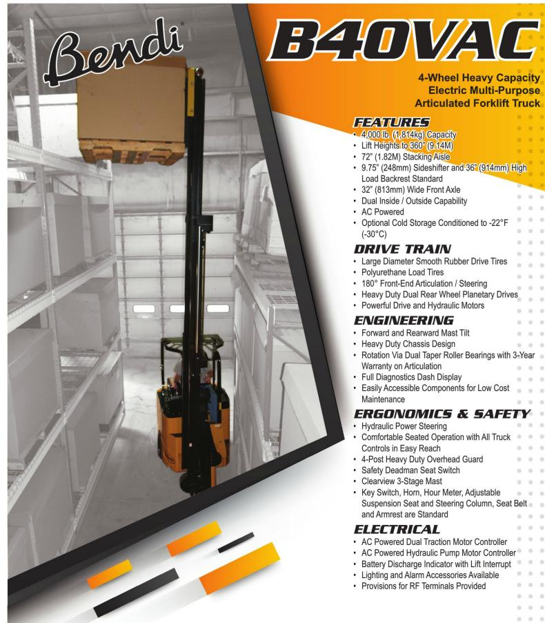
4-Wheel Heavy Capacity **Electric Multi-Purpose Articulated Forklift Truck**
