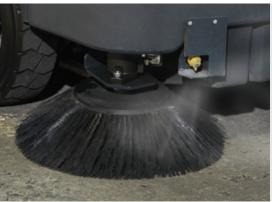
DustGuard™ suppresses airborne fugitive dust where most dust is generated – at the side brooms.
