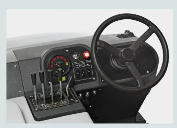
Ergonomic operator interface uses Analog-logic™ which allows a singe operator motion to lower and activate the main broom and side brooms and open the hopper door.
