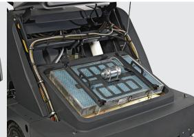
Patent pending Liberator<sup>™</sup> Variable Frequency Filter Shaker System removes dust more effectively from the panel filter, resulting in better air flow and dust control.
