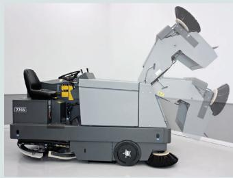
All-steel, 16 cubic foot debris hopper has a variable 60 inch dump system.
