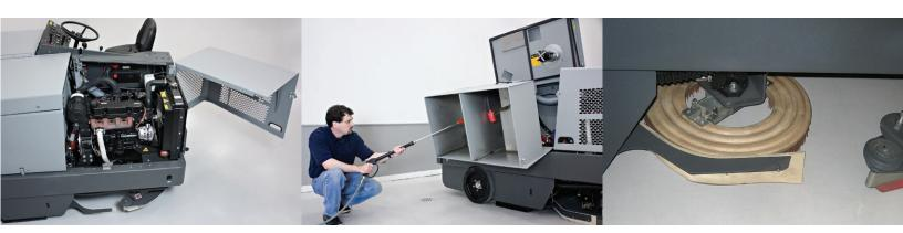
Maintenance is a breeze with easy-toreach engine, electrical and hydraulic components. Recovery tank tilts out for quick and easy clean-up, reducing the amount of time needed for draining and refilling.
