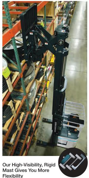
Achieve greater productivity with the SRX Series' high-visibility mast. Its rugged construction features **two interlocking I beam rails** nested within a rigid outer channel, and includes **six heavy-duty rollers** from carriage to mast rail.
